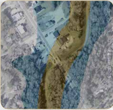
Above Left: The floodplain impacting the proposed Guignard Drive Node. Orange indicates the actual floodway, where development is not permitted. The photo ( above right ) indicates the presence of stormwater and poor drainage issues at this time. This photo was taken several days after a heavy rain.
