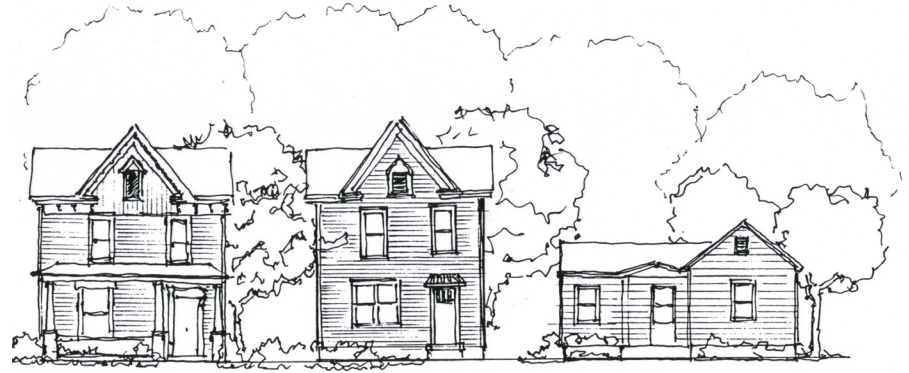
The one-story infill in the example above does not relate to the predominant heights or widths of surrounding buildings on the block.
